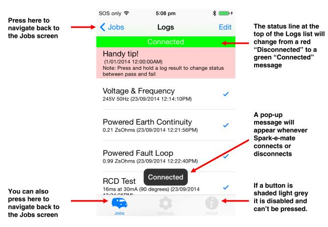
It's important to remember that <u>you must select a job and be in the Logs screen before</u> <u>Spark-e-mate will connect.</u> If you navigate away from the Logs screen Spark-e-mate will disconnect.
