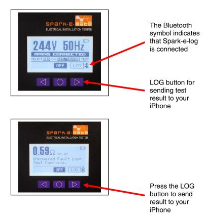
Both Spark-e-mate and your iPhone will beep to indicate successful data transfer. The test result appears in the Logs screen and is saved in Spark-e-log's database.
