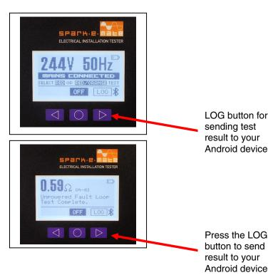
Please note that if you log the mains voltage and then perform a fault loop test, Spark-e-Log will automatically calculate and log the Prospective Short Circuit Current (PSC).
