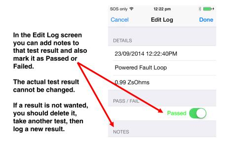
**Tip:** A quick way to mark a log result as Passed or Failed is to <u>push and hold</u> a log entry for one second.
